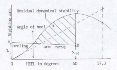
Note 1:  $\lambda_0 = \frac{\text{volumetric heeling moment}}{\text{SF x Displacement}}$
