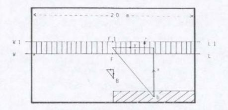
BMT = I\*COF intact water-plane  $\div$  volume =  $\frac{LB^3}{12V} = \frac{200 (20^3)}{12(32000)} = .4.167$  metres.
