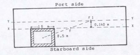
After bilging & parallel sinkage, the area of the water-plane is constant at all drafts. So F1 & B1 will be in the same vertical line and the new KB will be half the new draft. New KB = 4.132 m.
