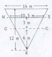
z = Depth of COP below ws = 4.500 m Sounding ... ... = 9.000 m KP (height of COP above bottom) 4.500 m
