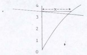
At each station, such area, multiplied by a length of one metre and by 1.025 would give the buoyancy per metre, in tonnes. The buoyancy curve can then be drawn to scale with the LOA as the base.
