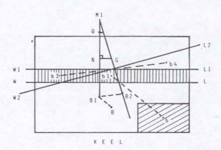
B<sub>1</sub> is the COB after bilging and parallel sinkage. Note: BB<sub>1</sub> is parallel to bb<sub>1</sub>.
