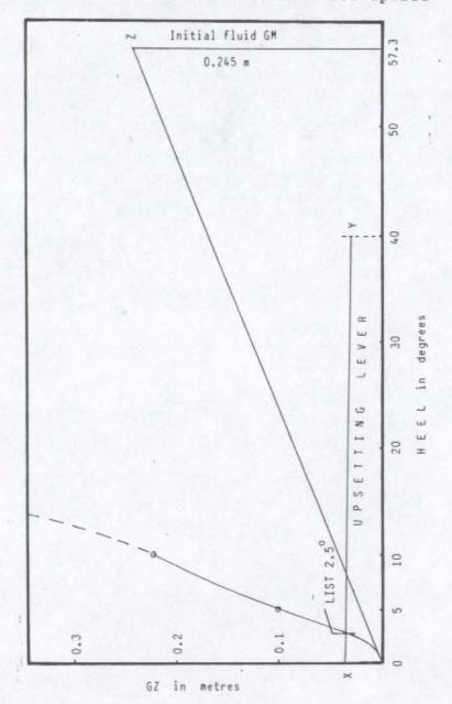
to arrive at point Z. Pdint Z and the origin are joined by a straight line &, while drawing the curve of statical stability, it is ensured that the curve coincides with this line for the first few degrees. It is this technique that makes method 1 a little more accurate than method 2.
