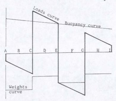
In the above diagram, a larger scale has' been used for the loads curve than for the curves of buoyancy and weight. The values of SF at each point:
