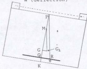
The GM for each shift of weight is calculated and the average initial fluid GM, in that condition, is obtained. The actual method of averaging varies between shipyards. Some average the deflections to port and starboard for the same weight shift. Some shipyards prefer to use weights of different values.
