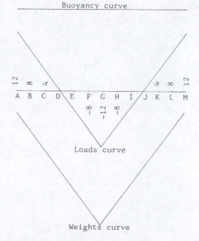
Calculating the area under the loads curve, the SF at each point is as under:
