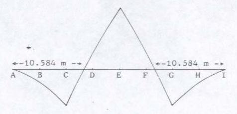
By using Simpson's first and third rules and plane geometry:
