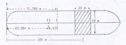
From hydrostatic table, at 5.325 m draft in salt water, assuming hull to intact:
