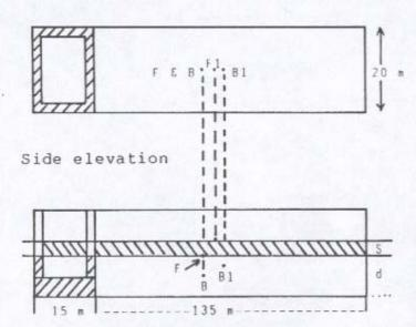
$V = 150 \times 20 \times 8 = 24000 \text{ m}^3$ ) Unchanged W = 24000(1.025) = 24600 t) by bilging
