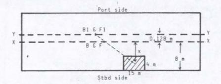
After bilging & parallel sinkage, the area of the water-plane is constant at all drafts. So F1 and B1 will be in the same vertical line and:
