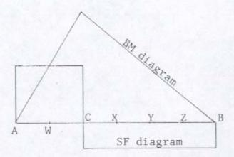
Note: The SF curve consists of two horizontal straight lines. So the BM curve consists of two sloping straight lines, as mentioned earlier in this chapter.
