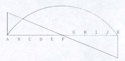
After drawing the SF curve, the values of BM may be computed, as described earlier in this chapter, and the results obtained, in kN m, would be:
