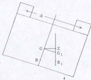
In the above figure, B & G are the initial positions of the COB and the COG. G<sub>1</sub> is the position of the COG after the transverse shift of weight.
